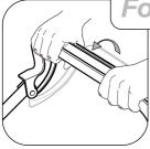
**Push Models** - Hold and push against the handlebar with both hands to move the mower forward.
